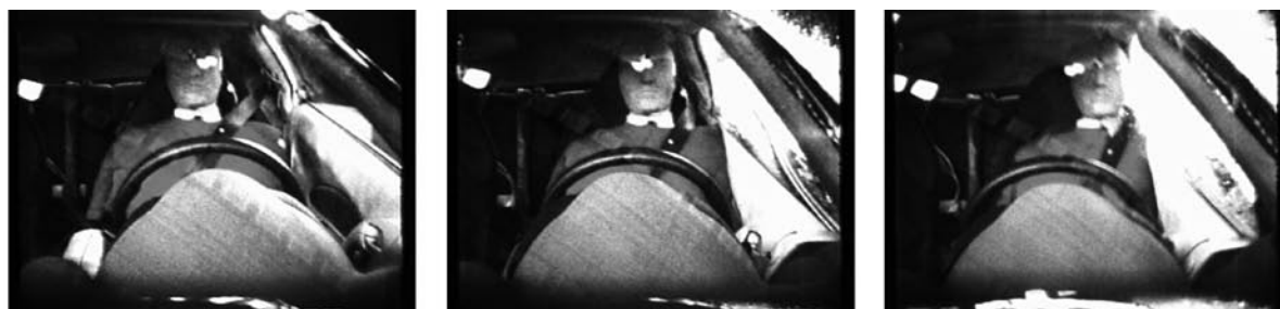
Figure 1: Example of the door punch mechanism from NCAP test, left, just prior to impact, center, door contacts shoulder, right, door contact dummy along side, dummy is still in upright position.
