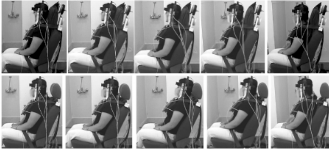
Figure 2: Test subject on sled with headband and chest plate containing accelerometers. Upper, modified head restraint, lower, the same subject with the standard head restraint. Note gap between head and head restraint in lower sequence (Time of images, from left to right, impact, 0 msec, 33 msec, 66 msec, 132 msec).
