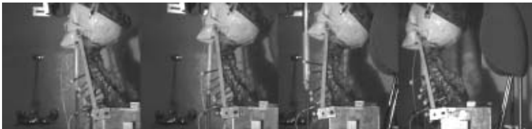
Figure 4: Cadaveric cervical spine responses from left, at 1, 88, 144, and 228 msec. Note lower to middle cervical spine extension at 144 msec and flexion at 228 msec.
