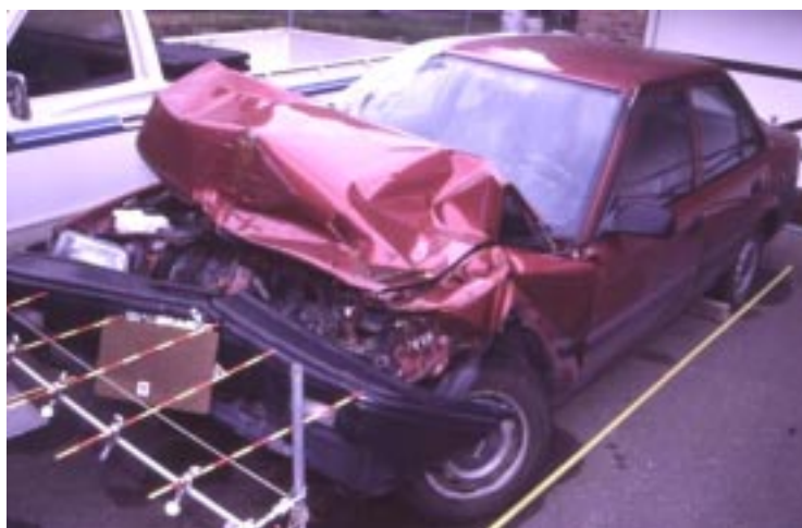
Figure 1: Vehicle in which the driver sustained the femur fracture of Figure 3 through contact with the dashboard, shown in Figure 2. This was a direct frontal collision with a speed change about 25 mph. The dashboard and interior surfaces remained intact and were not pushed towards the driver's legs.
