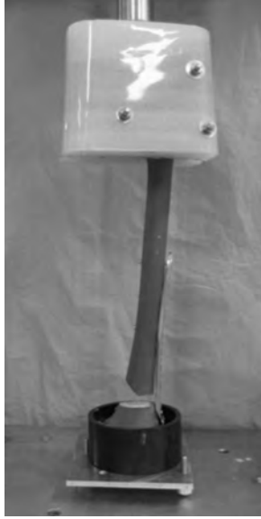
Figure 5: Set-up for axial loading. Distal segment mounted on platform with ball bearings to eliminate torque during loading.
