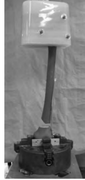
Figure 6: Set-up for torsional loading. Distal segment clamped into vice to introduce torque.
