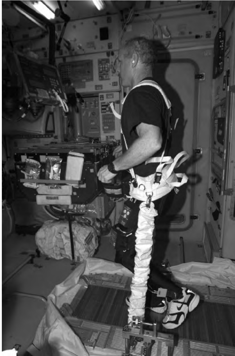
Figure 1: Astronaut running on a tethered treadmill on the ISS while wearing a set of instrumentation that we devised to measure joint motion, muscle activity, and ground reaction forces.
