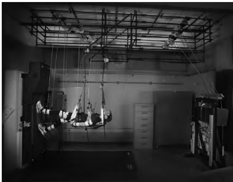
Figure 3: The Zero Gravity Locomotion Simulator (ZLS) on which bedrest subjects are exercised to simulate exercise during spaceflight.
