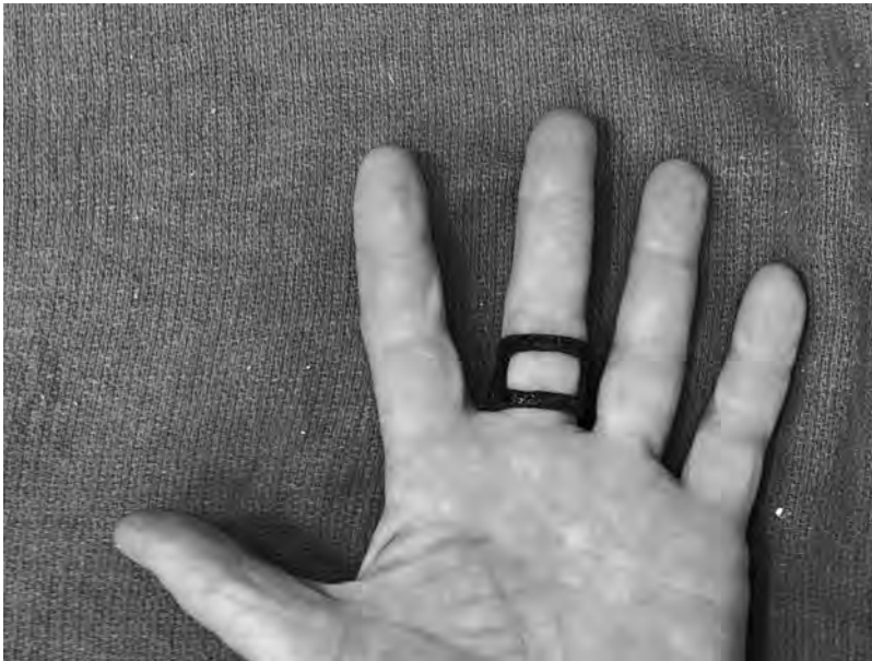
Figure 1: (A) Custom SPOrt. (B) SPOrt with window for ultrasound testing correctly positioned on a finger.
